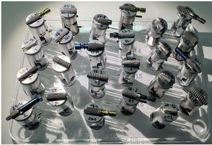
Fig. 2: Sterile implants mounted on a sample holder waiting for SEM analysis.
