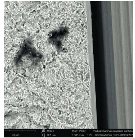
Fig. 3: Organic contaminants on the entire implant shoulder – identified as silicone-containing plastic residues (polysiloxanes) byToF-SIMS.
